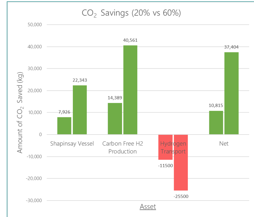
CO 2 savings achieved from hydrogen injection system for 20% and 60% displacement levels
